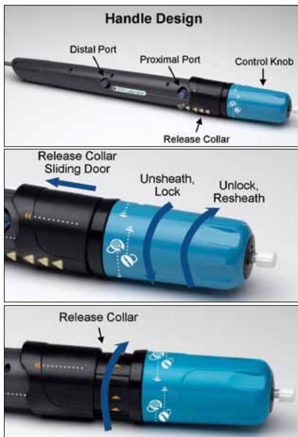
Figure 2. Delivery system handle design. The handle consists of two components: the control knob (blue), which unsheaths and locks the valve when rotated counterclockwise or unlocks and resheaths the valve when rotated clockwise, and the release collar, which releases the valve from the delivery system with clockwise rotation. The handle design ensures that the sheathing, locking, and release steps are performed in the appropriate sequence. Positioning of the valve can be adjusted at any point up until the final release.
